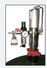
Prevents quick coupler from making a connection while locked.
