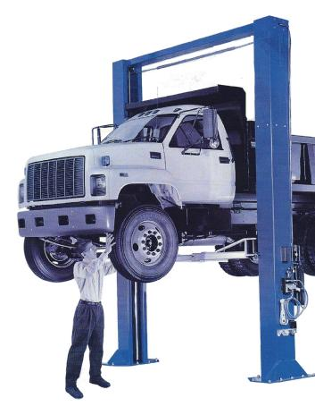
This power unit is designed specifically for use on 2 and 4 post auto hoists. This is for raise-hold-lower of the lift, with manual control of the lowering speed. A push-button, mounted on the unit, starts the motor to raise the lift. The unit features a fixed releif valve, so the lift cannot be overloaded, but(depending on cylinder size) can be used on most 7000 to 9000 lbs. capacity lifts.
