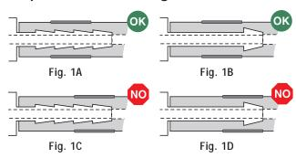
In the illustrations above, the clamps are properly positioned in Figure 1A and 1B, directly over the middle barbs and behind the first barb. This is extremely important in the case of single-barb fittings, as shown in Figure 1B, since the barb is generally much larger than the shank of the fitting. The compressed material cannot pass over the barb when under tension, thus securely holding the fitting to the hose.
