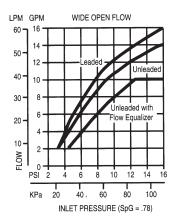
Standard Flo-Equalizer regulates flow to 10 GPM max.
