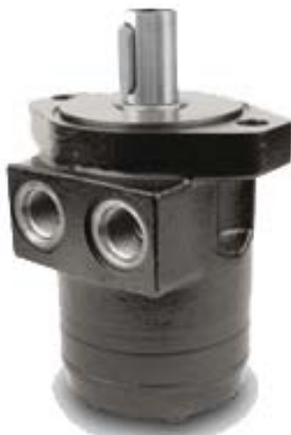
WG motors incorporated a needle bearing to provide and especially solid platform for any medium duty application where side load may present a concern.
