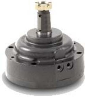
BK brakes provide up to 10,000 lb-in. of holding torque. This compact spring-applied, hydraulically released brake eliminates the cables, linkages, cylinders and brackets used in other brake systems, providing a simpler, more cost-effective solution.
