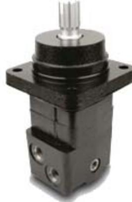
WS motors feature a robust design for medium duty applications and high flow rates--a three zone commutator valve for higher flow capacity; heavy duty tapered roller bearings for increased side load; and a larger drive link to better withstand pressure and torque spikes.
