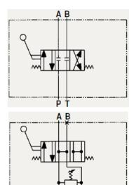
Rotary Spool Three-Way Closed Center no Relief Valve
