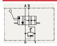
Rotary Spool Three-Way Tandem Center with Relief Valve MODEL NUMBER 20048-1/2" NPTF Ports 20049-3/4" NPTF Ports (SAE ORB Ports also Available)
