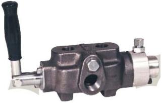
The valve handle is rotated to actuate the spool, as opposed to shifting the spool axially. This provides finer metering control. These valves incorporate a mechanical detent in the neutral position.
