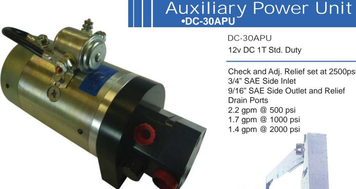
The power unit is intended to be used with remote directional control valving and reservior. This unit has an adjustable relief valve and outlet check valve. They are designed for applications such as backup (auxiliary) hydraulic power for truck mounted or the other mobile equipment, including emergency power steering for offhighway vehicles, elevated platforms, aerial buckets and manlifts. It can also be used to power material handling functions and other intermittent duty
