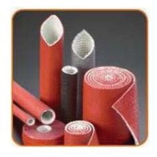
Designed to protect hoses, wires and cables from the hazards of high heat and occasional flame. It protects continuously to 500°F and will withstand a molten splash at 2200°F. Made of either knitted or braided fiberglass yarns in a flexible substrate that is then coated with high-grade silicone rubber.
