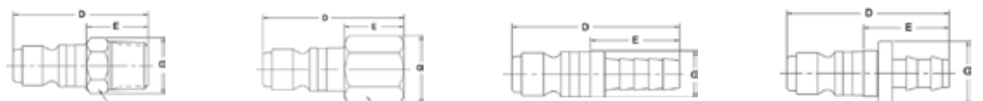
Male Thread Nipple Female Nipple Hose Barb Nipple Push Lock Hose Barb Nipple
