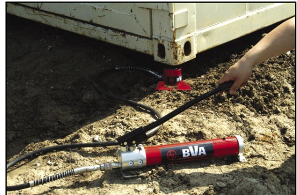
• Low profile cylinders are great for confined spaces
