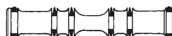
2 Position 90A20225 - Aluminum Spool - Mechanical Operators 90A20226 - Plastic Spool - Solenoid and Air Operators
